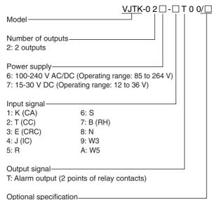
Blank: With socket /SN: Without socket
